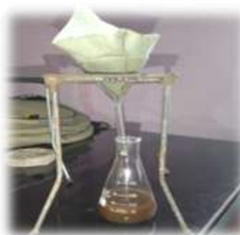
Fig 8: Filtration of concentrated extract
